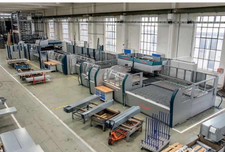
Connected arrangement of a MD storage tower, a S4Xe combined punching shearing and P4lean bending unit Picture: Meiller
